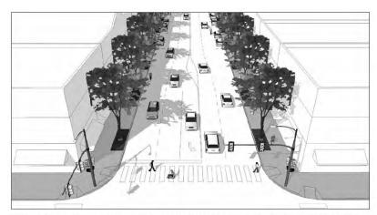
**Figure 4.6** Illustration of an avenue. In this example on-street parking is dropped to gain width for a left turn lane at the intersection. Source: Claire Vlach, Bottomley Design & Planning.
